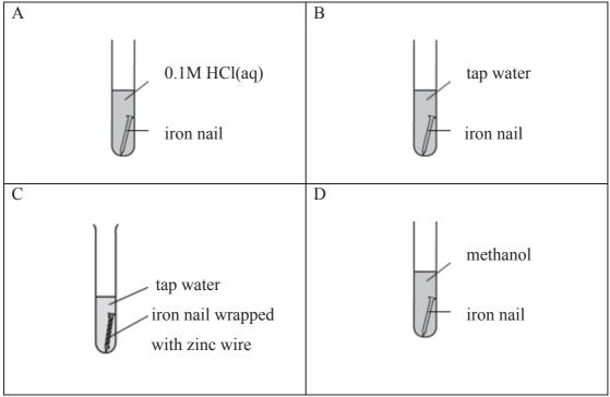
After some time, the solution from each tube was tested with potassium hexacyanoferrate(III) solution. It was found that corrosion of iron occurred only in tubes A and B.
